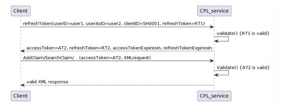
To refresh the accessToken AT1 the refreshToken() must be used. The refreshToken() RT1 can be used both before and after the expiration of the accessToken.
