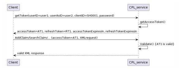
Together with the accessToken the getToken() functionality returns a field called refreshToken, this token must be used in the refreshToken() functionality to refresh the accessToken, the validity of this token is 86400sec (24 hours), (see paragraph **Errore.** L'origine riferimento non è stata trovata.)
